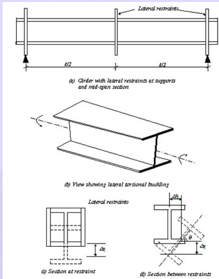
**Fig.7.18 Distorsion caused by lateral torsional buckling**
